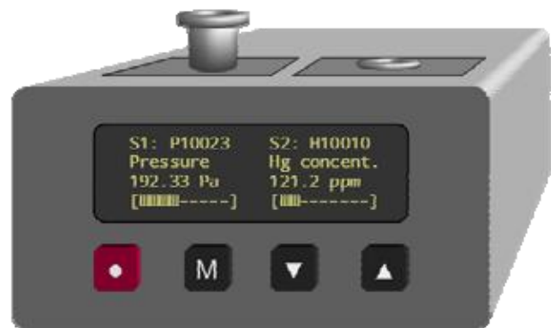
Picture 3. Conceptual rendering of the portable multifunctional instrument with two sensor modules installed
