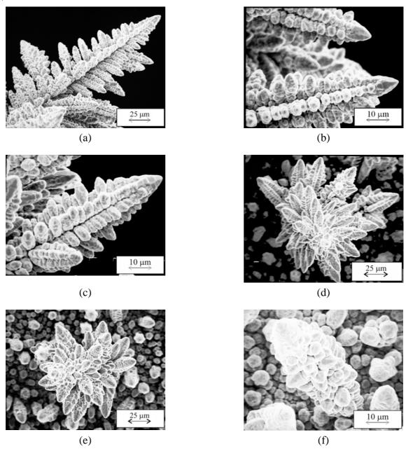
**Figure 7.** Copper deposits obtained at overpotential of 800 mV. Quantity of electricity: 10.0 mAhcm<sup>-2</sup>. (a) and (b): *solution (I)*. Magnification: (a) x 150, (b) x 5000; (c) and (d): *solution (II)*. Magnification: (c) x 150, (d) x 750; (e) and (f): *solution (III)*. Magnification: (e) x 150, (f) x 750.
