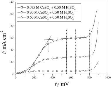
The effect of hydrogen evolution on copper electrodeposition was examined at overpotentials of 550, 650 and 800 mV. For all examined solutions, overpotentials of 550 and 650 mV corresponded to the plateau of the limiting diffusion current density, while an overpotential of 800 mV was about 50 mV outside the plateau of the limiting diffusion current density (Figure 1 and Table 1).
