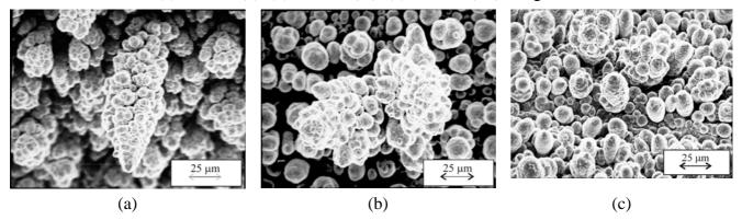
Figure 7 shows the morphologies of copper deposits obtained at an overpotential of 800 mV with a quantity of electricity of 10.0 mAhcm<sup>-2</sup>, which reveals the strong effect of concentration of Cu(II) ions on copper electrodeposition at this overpotential.
