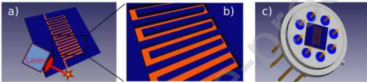
Fig. 1 The illustration of one part of the fabrication procedure, a) Direct laser writing, b) Zoom into the interdigitated structure, c) The illustration of the finished chip mounted on the TO-8 housing. The digits are enlarged in order to show the concept of the sensor.
