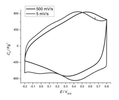
Fig.1. Cyclic voltammograms of nanocrystalline RuO<sub>2</sub> in 1 M H<sub>2</sub>SO<sub>4</sub>.
