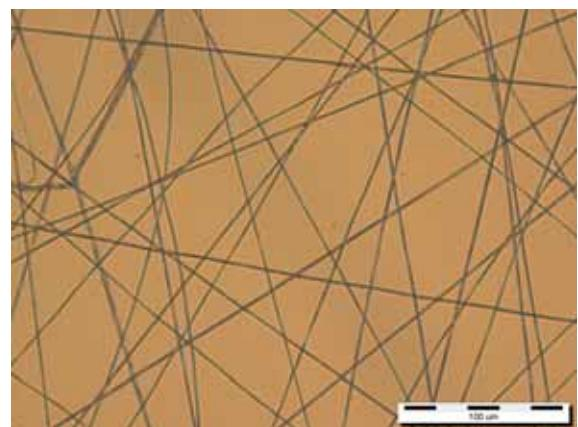
**Figure 5.** Optical microscopy image of the PVB fibers with 3 wt.% modified SiO<sub>2</sub> nanoparticles ( $Q = 1\text{mL/h}$ ,  $V = 20\text{kV}$ ,  $h = 10\text{cm}$ )
