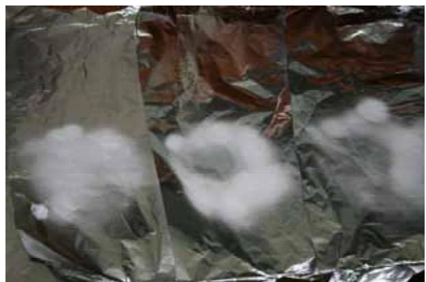
**Figure 4.** The collected nanofibers on the aluminium foils
