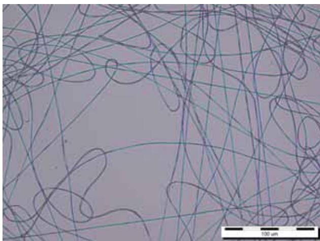
**Figure 6.** Optical microscopy image of the PVB fibers with 3 wt. % unmodified SiO<sub>2</sub> nanoparticles ( $Q = 1\text{mL/h}$ ,  $V = 24\text{kV}$ ,  $h = 10\text{cm}$ )
