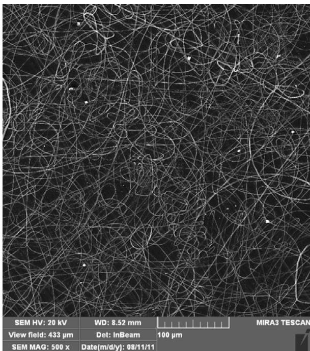
Figure 10 - SEM photograph of the PVB fibers with 1 wt.% unmodified SiO<sub>2</sub> nanoparticles (Q = 1mL/h, V = 30kV, h = 10cm)
