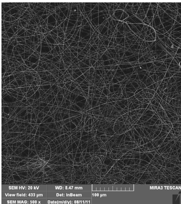
Figure 11 - SEM photograph of the PVB fibers with 1 wt.% modified SiO<sub>2</sub> nanoparticles (Q = 1mL/h, V = 30kV, h = 10cm)
