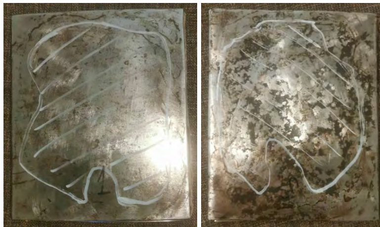
Figure 9. Explosively welded plates 1 and 2: area of weld, registered by ultrasonic method.
