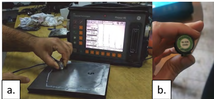
Figure 3. a) Ultrasonic thickness measurement of Explosively Welded joint b) SE probe
