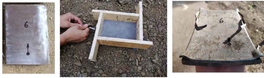
a) Plate before welding, experimental set-up with Amonex explosive, and welded plate Al/Steel
