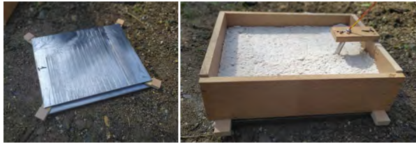
b) Left: steel plates in parallel configuration with wooden spacers; right: wooden frame placed over the plates with DEMEX explosive and blasting cap placed in a holder
