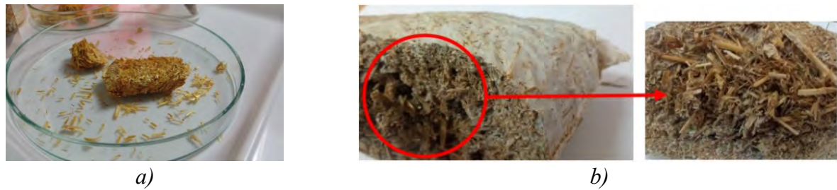
Figure 1. Realization of a biocomposite block based on mycelium: a) straw base, b) realized composite showing different granulation and distribution of fillers
