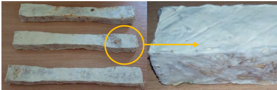
Figure 5. Biocomposite specimens with an enlarged view of the mycelium sheath
