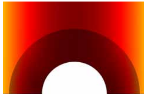
Picture 7: Total acoustic pressure map at a cylindrical scatterer surrounded by multilayered shell, 20 Hz. Highest pressure is 1 Pa (dark red), lowest 0.95 Pa (dark blue)
