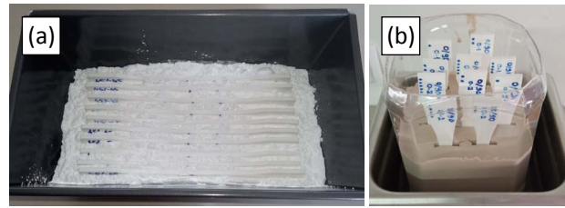
Figure 3. Specimen moulding: (a) in NaCl powder and (b) in plaster
