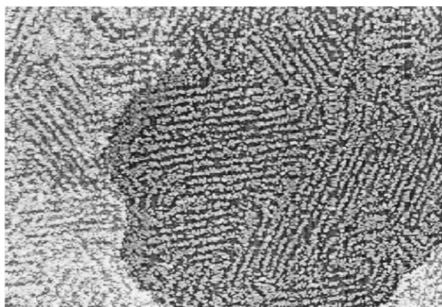
FIG. 4. STM image recorded on Au(111) in 0.5 M \text{H}_2\text{SO}_4 at 0.0 V after deposition of 0.30 ML from 0.5 M \text{H}_2\text{SO}_4 + 10^{-4} M \text{RuCl}_3 at 0.0 V ( 3200 \times 2200 \text{ \AA}^2 ).
