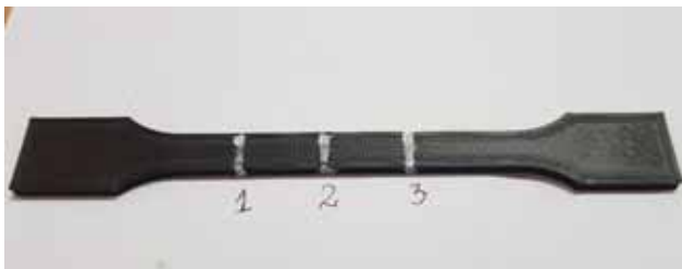
Figure 8. Measured location of the FDM specimen
