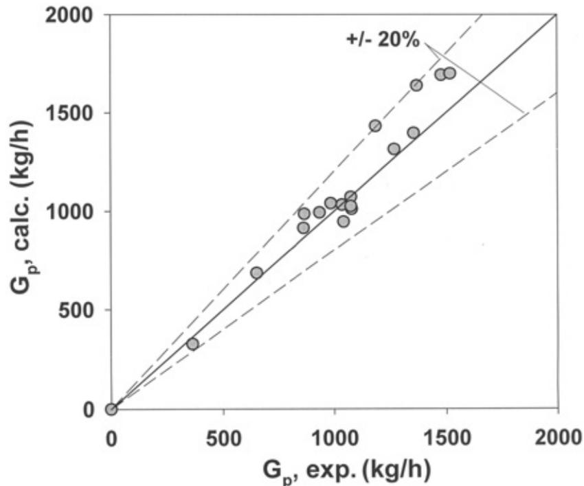
Fig. 3. Comparison between the calculated and measured values of the particle circulation rate.
