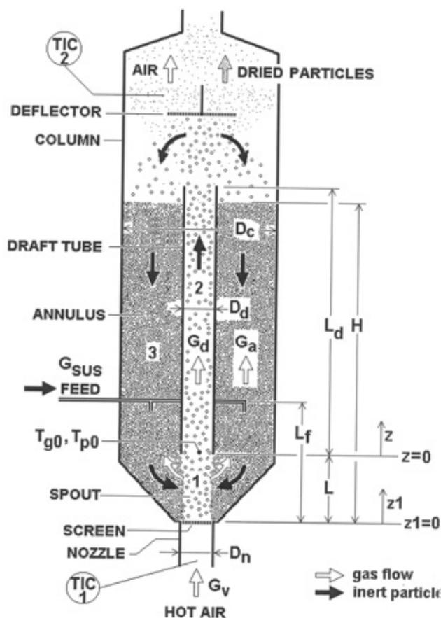
Fig. 1. Schematic diagram of the draft tube spouted bed dryer (DTSB).
