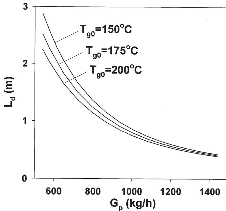
Fig. 2. The draft tube length required for complete evaporation as a function of the particle circulation rate and the inlet air temperature ( $G_v = 306$  kg/h;  $G_d = 265$  kg/h;  $G_a = 41$  kg/h;  $T_{p0} = 73$  °C; feed-water,  $G_{SUS} = 12$  kg/h).
