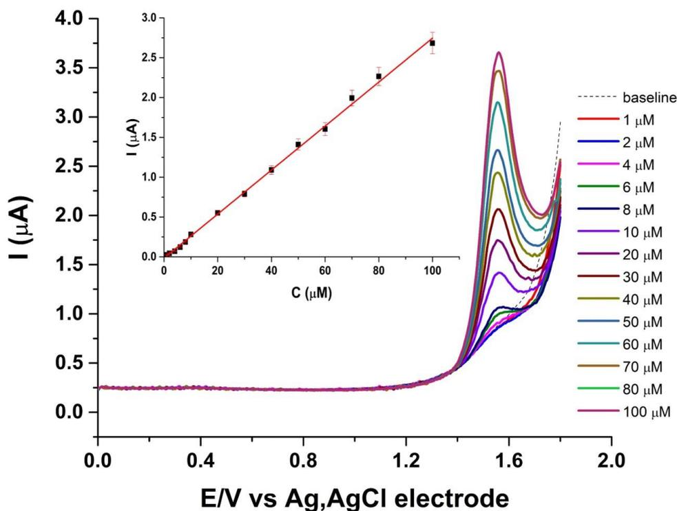
**Figure 5.** Voltammograms obtained for different concentrations of clomazone in positive potential range. SWV technique, working electrode BDD, reference electrode  $\text{Ag/AgCl}$  electrode, supporting electrolyte BRBS (pH 2). Pulse amplitude 40 mV, frequency 20 Hz. Insert figure shown corresponding calibration curve.
