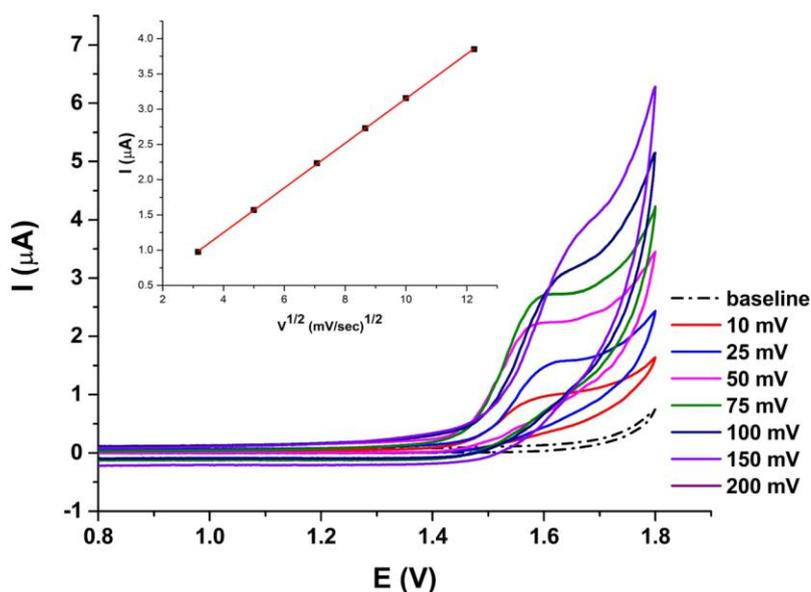
**Figure 3.** Cyclic voltammograms of 0.1 mM of clomazone at BDD electrode (working electrode) and Ag/AgCl electrode (reference electrode) in BRBS at pH 2 at various scan rates from 10 to 200 mV/s. Inset figure present dependence of the peak current from the square root of the scan rate.
