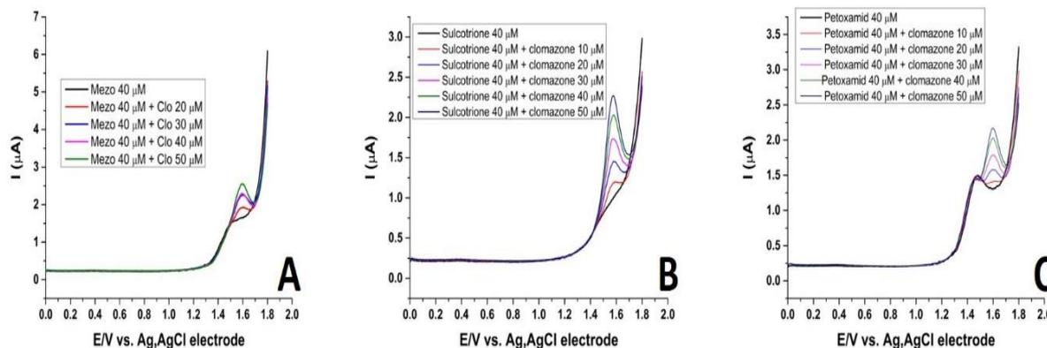
**Figure 6.** Electrochemical response of clomazone in the presence of some tested interferences by SWV method: A) mezo; B) sulcotrione; C) pethoxamid. BDD as working electrode, Ag/AgCl electrode as reference electrode, supporting electrolyte BRBS at pH 2. Pulse amplitude 40 mV, frequency 20 Hz.
