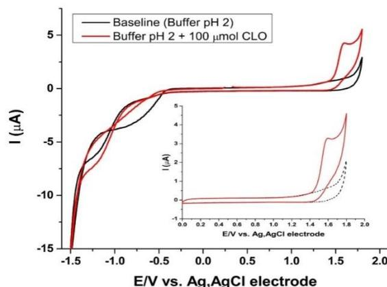
**Figure 1.** Cyclic voltammogram of 0.1 mM of clomazone in BRBS at pH 2 with BDD as working electrode and Ag/AgCl electrode as reference electrode. Scan rate 100 mV/s. Insert figure shown electrochemical response of 0.1 mM clomazone in anodic range potential.
